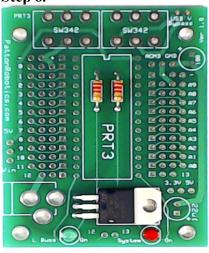
With care it is quite easy to get the hole on top of the voltage regulator to align with the hole in the circuit board. When aligned, solder in the voltage regulator and trim off the excess wire.
