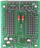
With the Patton Robotics logo facing up, insert two  $2.2k\Omega$  resistors into the circuit board as shown.
