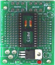
Being careful not to bend the tiny pins, insert the 28-pin socket into place on the circuit board. The notch in the socket should be nearer the top of the circuit board (opposite the voltage regulator) as shown. Once the board is in place, solder just one of the pins. Flip the board over to ensure the socket is lying flat on the board. If so, solder the remaining pins.
