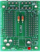
Next place the Red and Green LEDS into the board as shown. The board is oriented with the green LED on the left and the red LED on the right, which is the preferred placement. Be sure to match the flat side of the LED with the flat side of the white line trace on the board.
