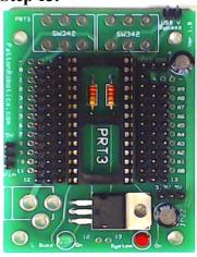
Insert the remaining rows into place as shown in the image at the left. (It may be a good idea to place and solder one or two rows at a time if you are not well experienced in soldering.) Be sure to insert the short ends into the board with the long ends sticking out of the board. It is important that the outer-most row of holes on each side of the board remain empty for now.
