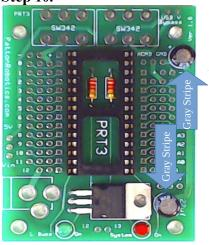
Insert the capacitors into the circuit board being sure that the  $100\mu F$  capacitor is nearest the edge of the board and the  $22\mu F$  capacitor closest to the voltage regulator. Carefully check that the capacitor's long positive wire lead is in the hole marked with a '+'. Double-check that the negative gray stripes on the capacitors are positioned as shown in the image. Once both are in place, carefully solder both to the board.
