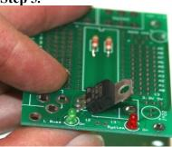
Soldering in the voltage regulator is best done in a few steps to ensure proper alignment. Start off by inserting the voltage regulator until it hits its wire stops. Make sure the front of the regulator (with the words) is facing the green LED. (The metal back of the LED should then be facing the red LED.)
