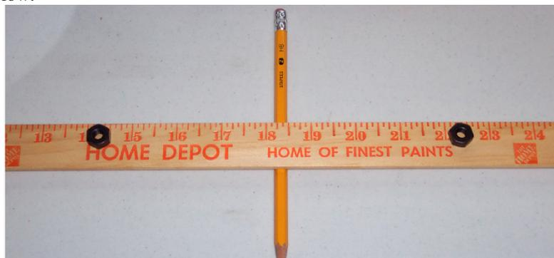
Slide the nut I tiny bit if you need to, but make sure the yardstick is balanced.
