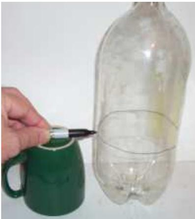
**Step 1:** Draw a line around the bottle about six inches up. I use a neat little trick to make a nice straight line. I rest the marker on the top of an upside down coffee cup then I rotate the 2 liter bottle. It makes a nice straight line.
